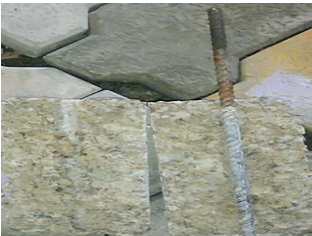
Fig. 3. Specimen representing concrete and reinforcement bar after pull out test.
