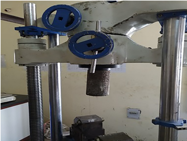
Fig. 2. Pull out test for treated lightweight concrete.
